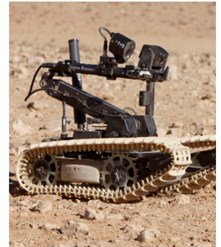
The lightweight Dragon Runner Bomb Disposal Robot is easy to transport and can be deployed in many different terrains (Crown copyright 2012)
